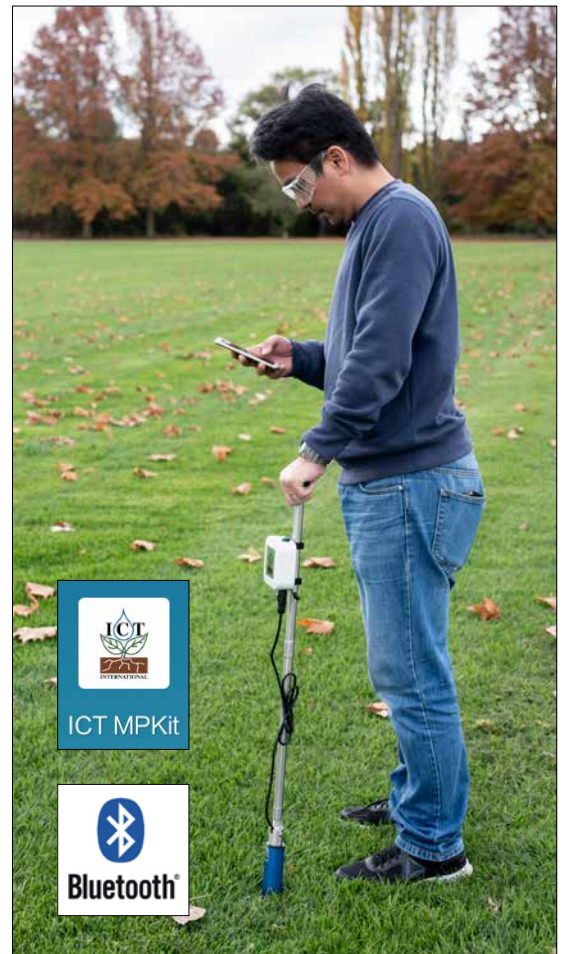
The MPKit Measuring Surface Volumetric Moisture Content for Managing Turf Grass
