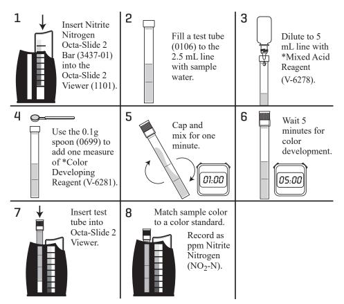
To convert to nitrite, multiply by 3.3. Record as ppm Nitrite. Nitrite-N (NO<sub>2</sub>-N) x 3.3 = ppm Nitrite (NO<sub>2</sub>-)
